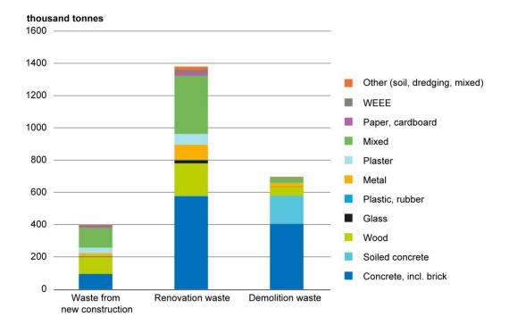
The most important types of construction waste until now have been concrete and wood waste, as well as the mixed waste mentioned above. Concrete waste is the largest waste
